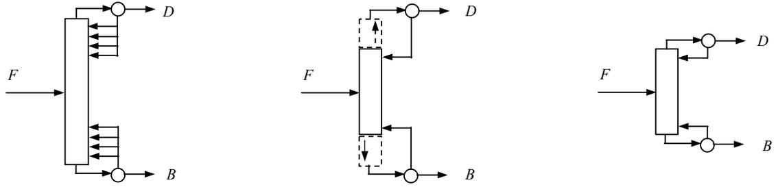
Figure 2: Variable reflux and reboil location with fixed heat exchangers
