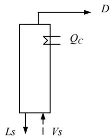
Figure 12: Lower boiler-rich distillate minimum energy demand calculation
