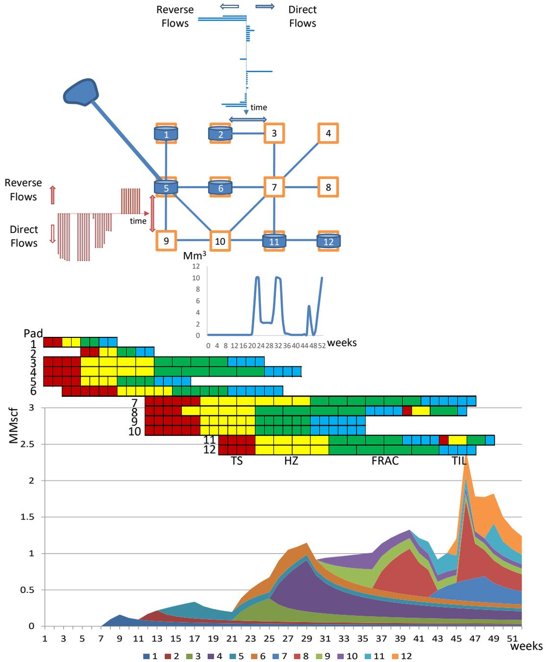
Figure 6. Optimal solution for the maximization of gas production revenues, and the most economical water distribution network required for complying with this development plan.
