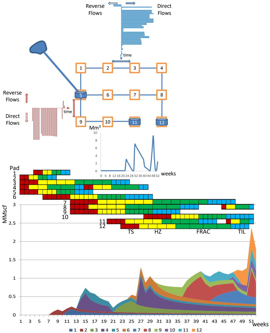
Figure 7. Best solution found for the simultaneous optimization of the wellpad development plan and the water distribution network design and operation.
