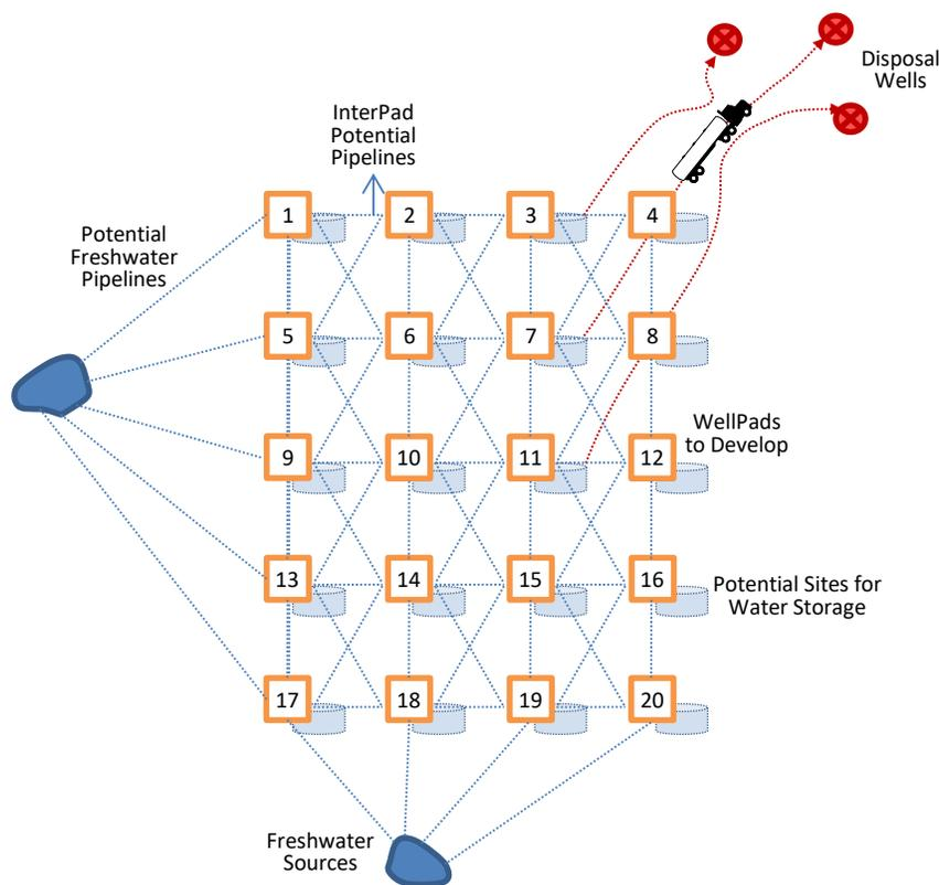
*Figure 1. Superstructure of Alternatives for the Design of Water Pipeline Networks over a Shale Gas Development Region*
