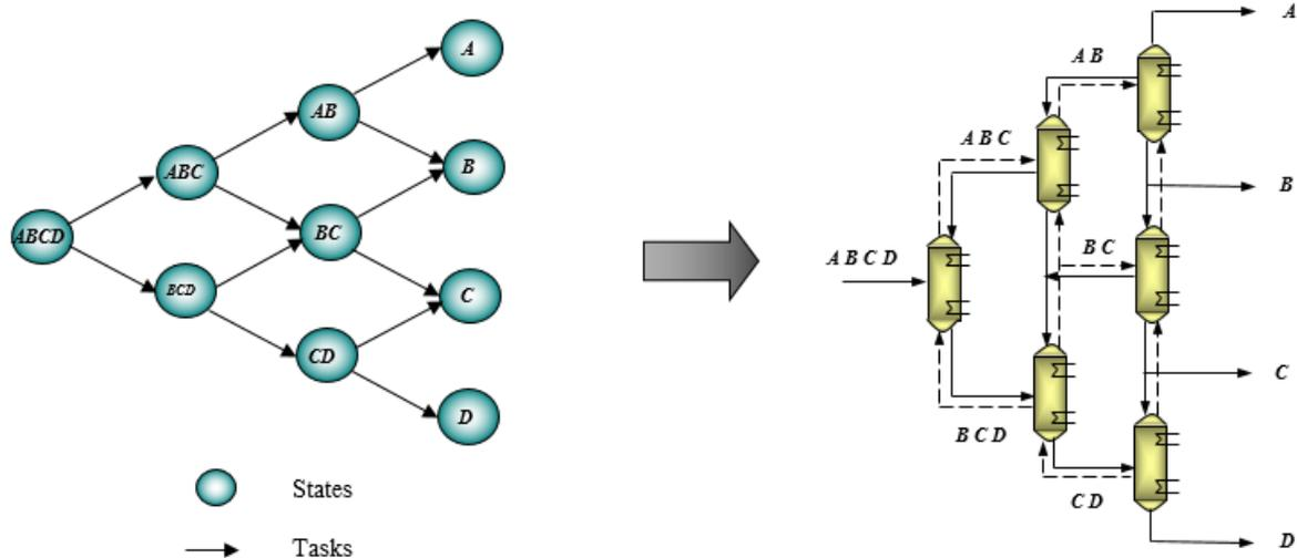
FIGURE 12: STN DISTILLATION SYNTHESIS SUPERSTRUCTURE FROM (195)
