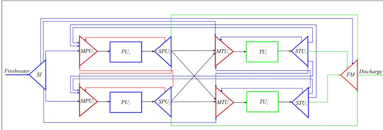
FIGURE 13: WATER NETWORK SUPERSTRUCTURE FROM (215)
