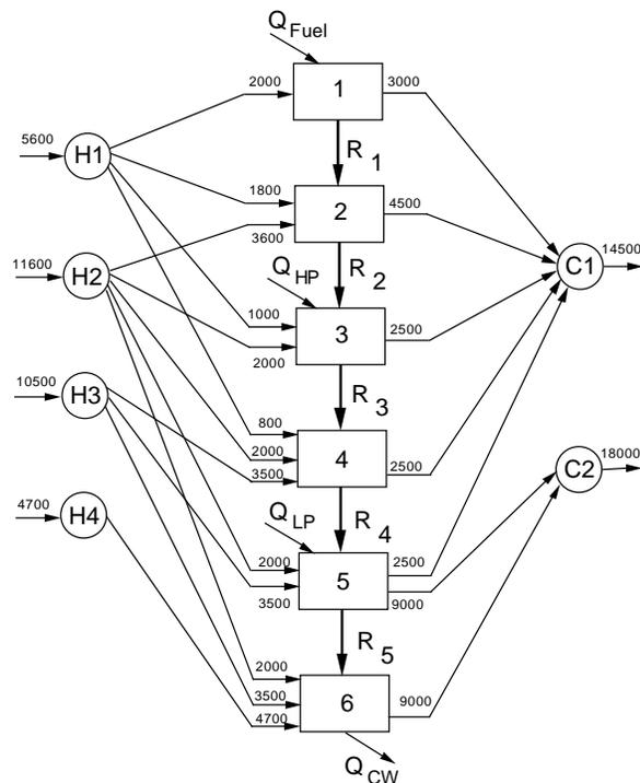
FIGURE 5: TRANSSHIPMENT LINEAR PROGRAMMING MODEL FOR HEAT EXCHANGE NETWORK SYNTHESIS
