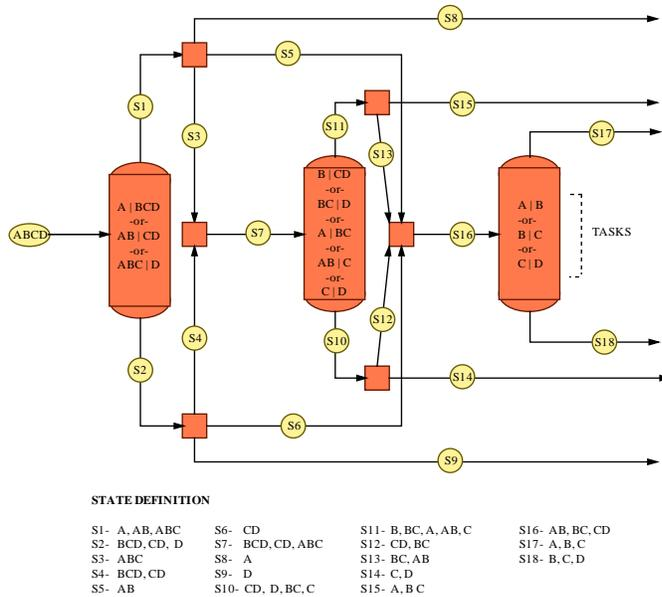
**FIGURE 4: STATE-EQUIPMENT NETWORK (SEN) SUPERSTRUCTURE, FIGURE FROM (72)**
