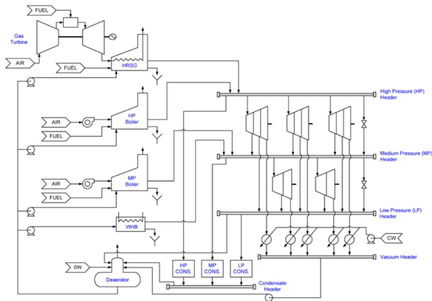
**FIGURE 11: UTILITY PLANT SUPERSTRUCTURE, FIGURE FROM (176)**
