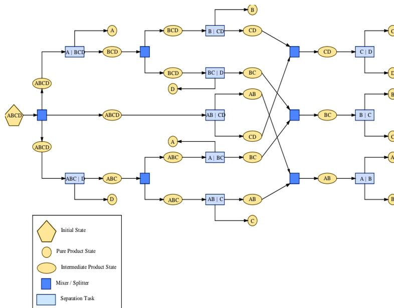
FIGURE 3: STATE-TASK NETWORK (STN) SUPERSTRUCTURE, FIGURE FROM (69)
