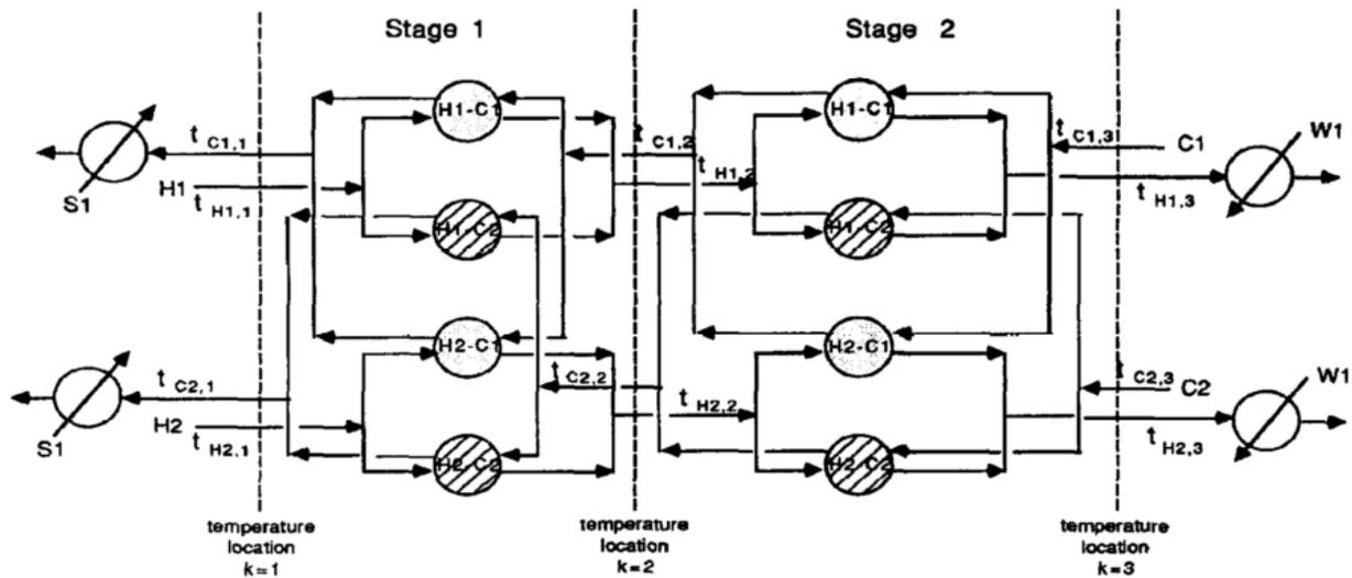
FIGURE 10: HEAT EXCHANGE NETWORK SUPERSTRUCTURE FROM (17)
