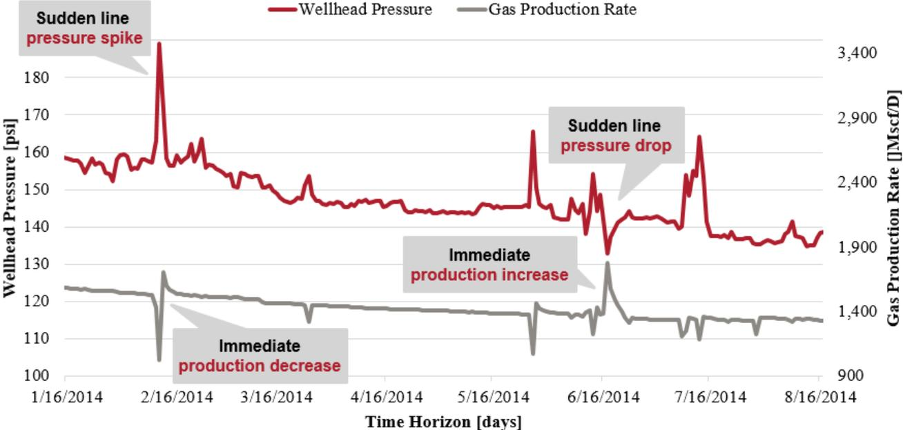
Fig. 2: Historic wellhead pressure and gas production rate of a single shale well over time
