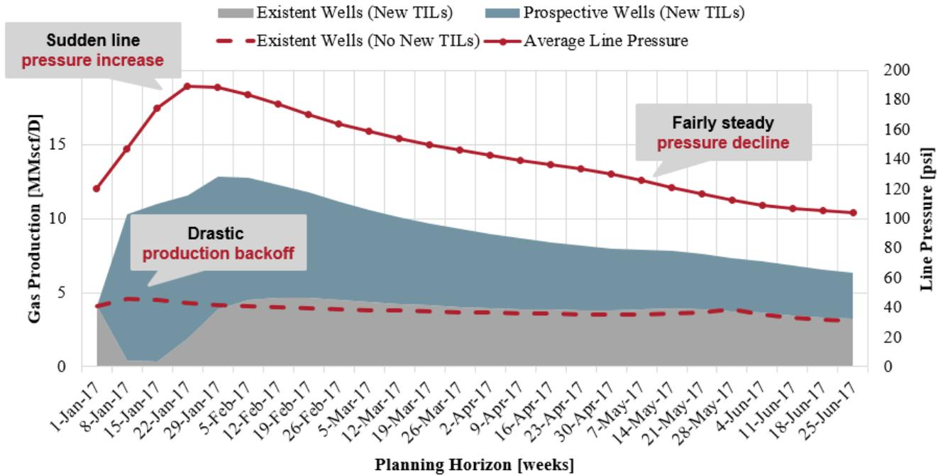
Fig. 3: Demonstration of the “backoff effect” in a shale gas gathering system when too many prospective wells are turned in-line at the same time
