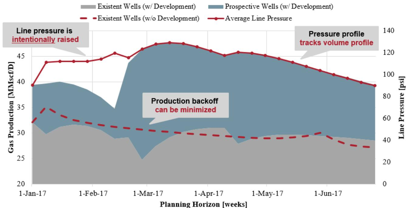
Fig. 11: Production volumes and line pressure over time distinguished by a) existent wells without development and b) existent and prospective wells with development
