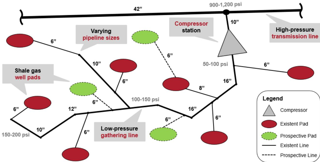
Fig. 1: Illustration of a typical shale gas gathering system with key network elements
