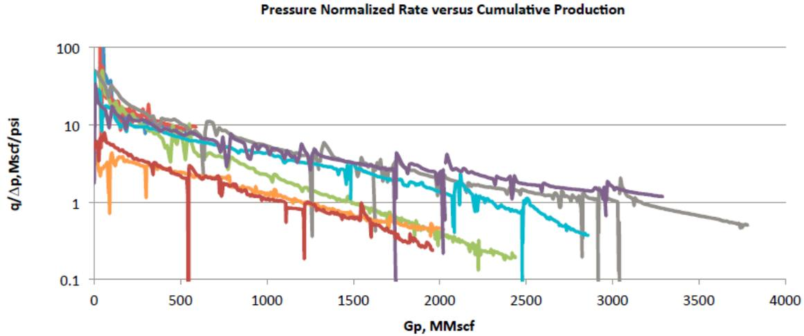
Fig. 4: Pressure normalized production rate over cumulative gas production for selected shale wells
