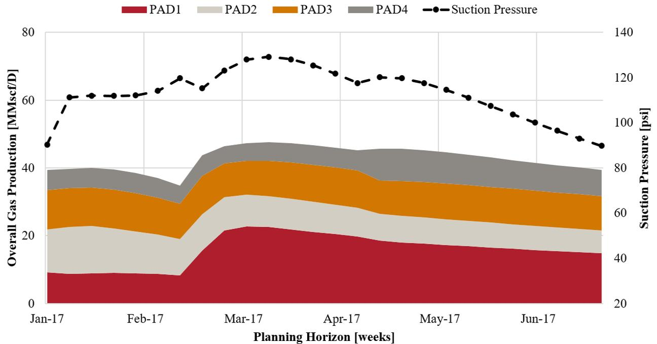
Fig. 9: Production volumes by pads over time compared to suction pressure at the compressor inlet
