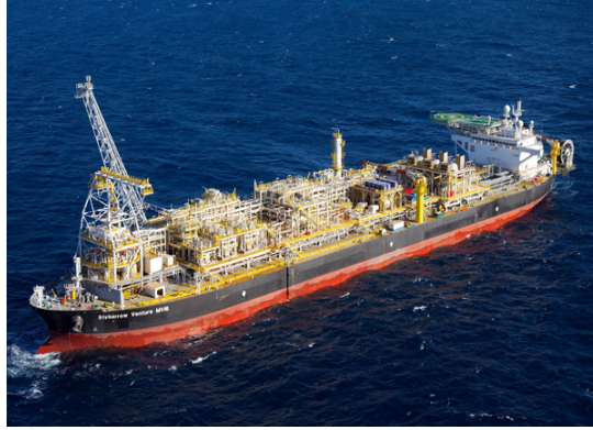
Figure 5: FPSO (Floating Production Storage and Offloading) facility
