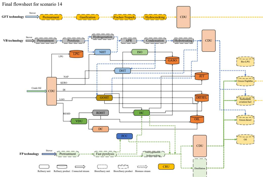
Fig. 12. Retrofitted flowsheet of the biorefinery for scenario 14.
