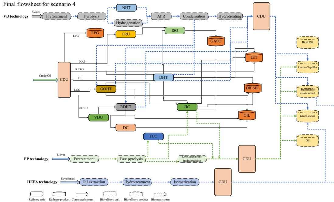
Fig. 11. Retrofitted flowsheet of the biorefinery for scenario 4.
