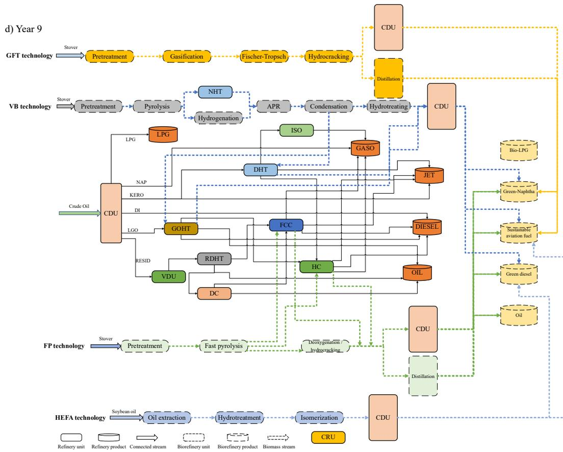
Fig. 6. Retrofitted flowsheet of the biorefinery over planned years.
