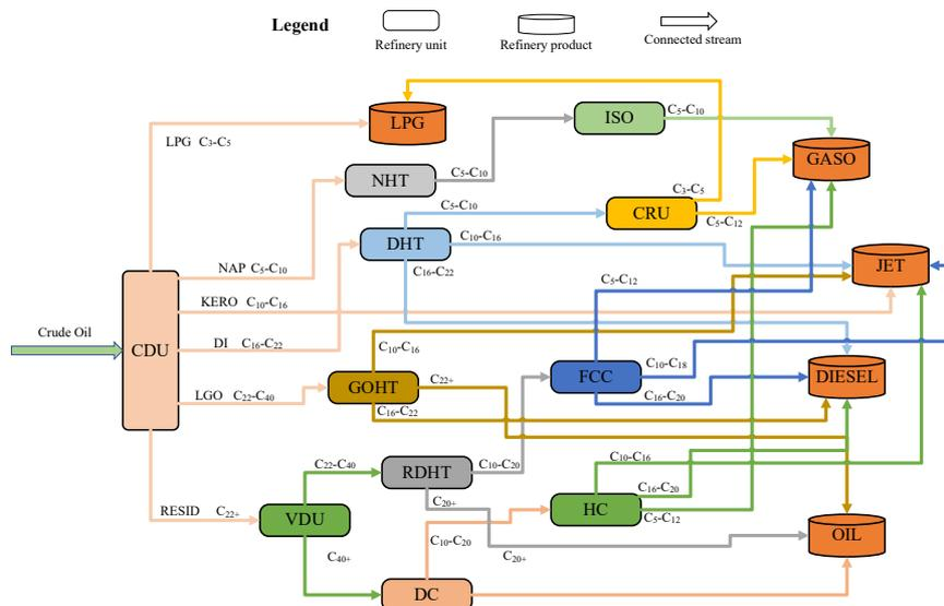
Fig. 1 Flowsheet of a given crude-based refinery.
