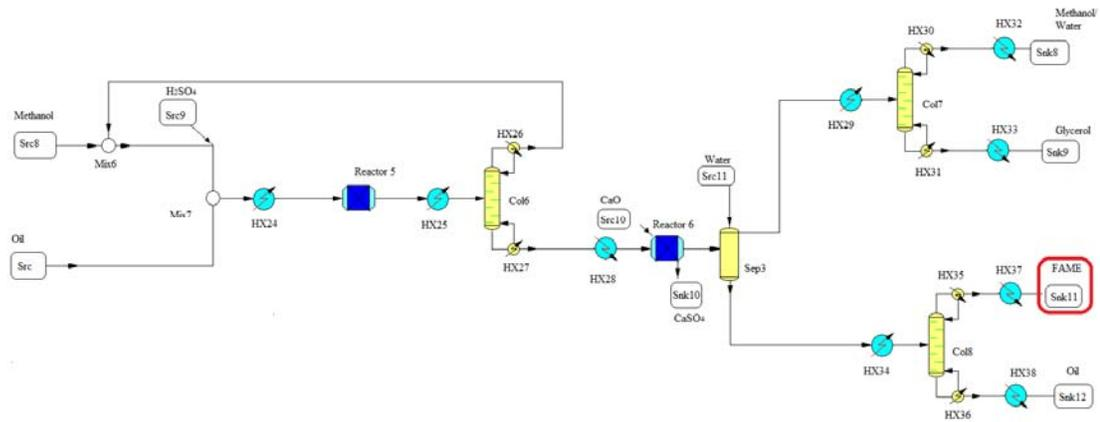
Figure 7.- Flowsheet for the production of biodiesel from oil via acid -catalyzed transesterification
