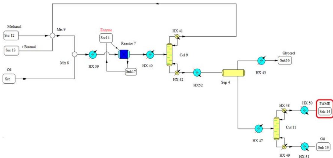
Figure 10.- Flowsheet for the production of biodiesel from oil via enzymatic transesterification
