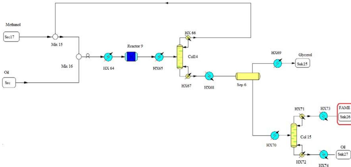
Figure 12.- Flowsheet for the production of biodiesel from oil via supercritical non catalyzed transesterification
