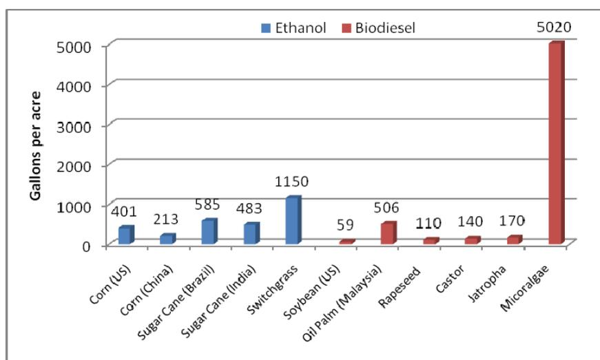
Figure 1.- Yield of biofuel for different raw material per area
