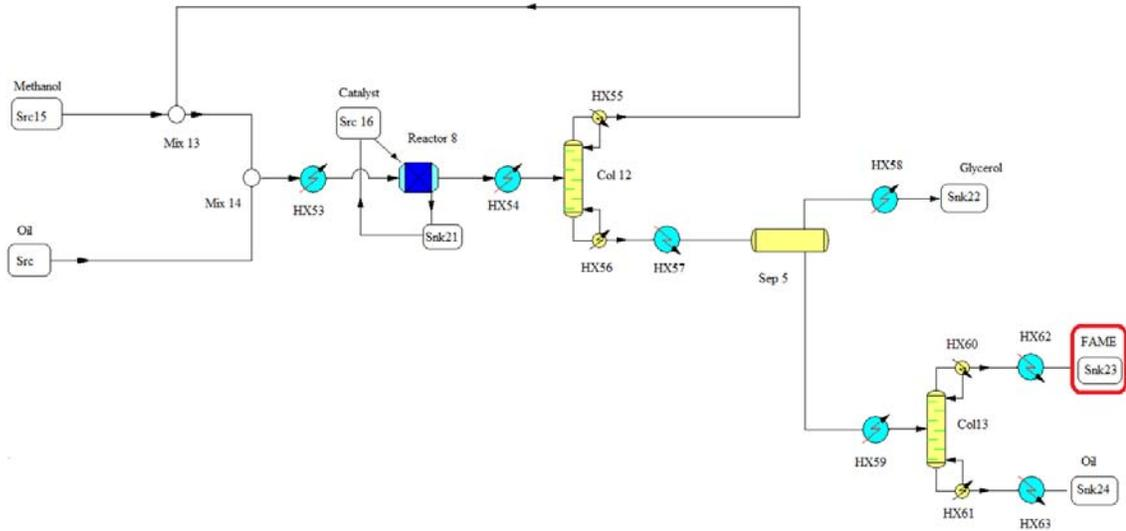
Figure 9.- Flowsheet for the production of biodiesel from oil via heterogeneous -catalyzed transesterification
