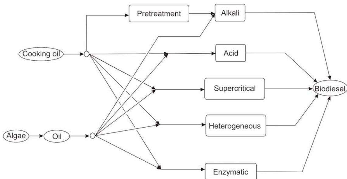
Figure 2 .-Supersstructure of alternative processes.
