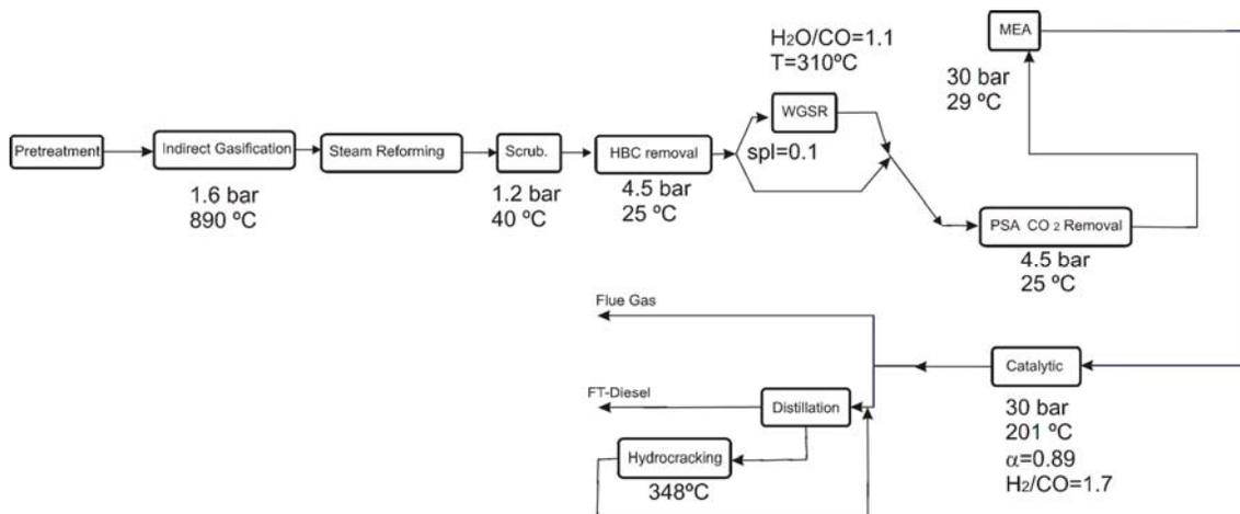
Figure 16. Optimal flowsheet( $H_2/CO_{min}=1.7$ )
