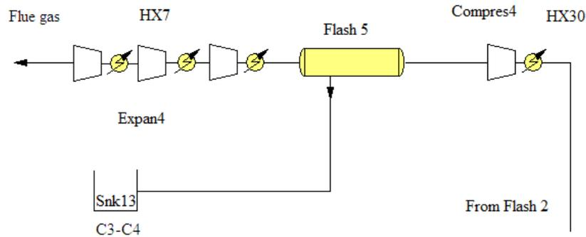
Figure 8. Gas treatment and separation
