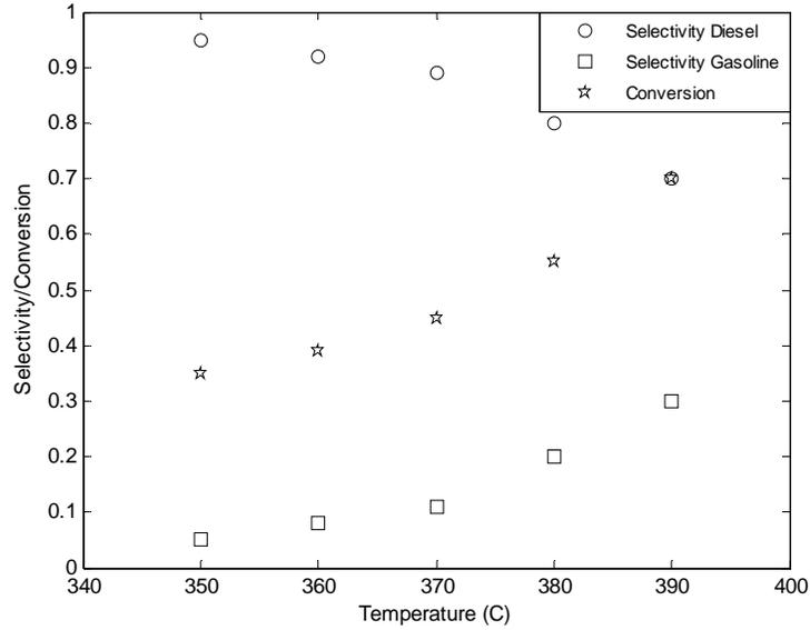
Figure 10.- Conversion profiles for the hydrocracking reactor
