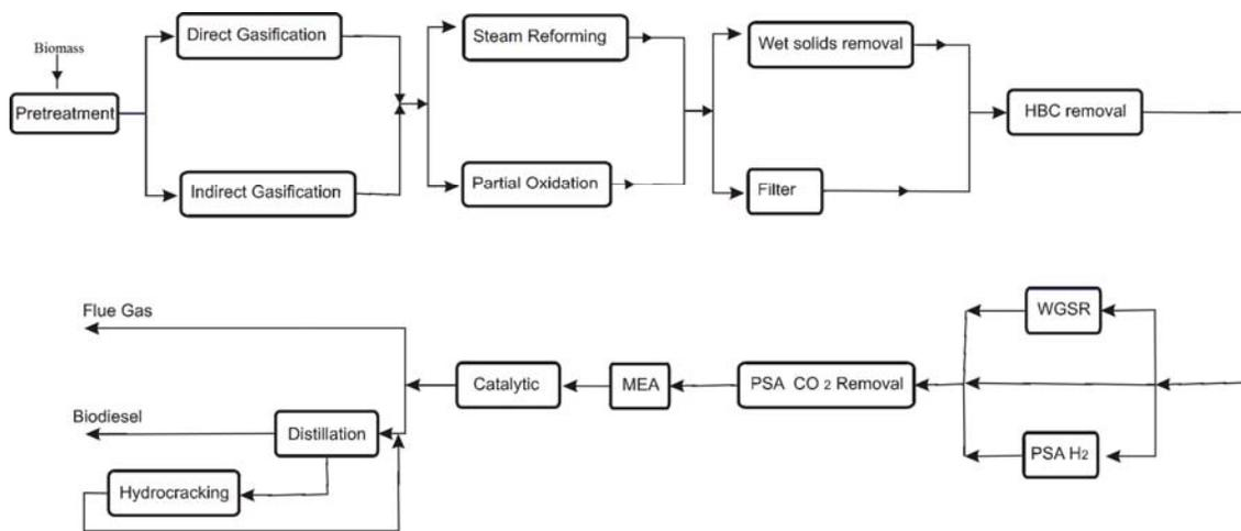
Figure 1.- Superstructure for the production of FT- Diesel
