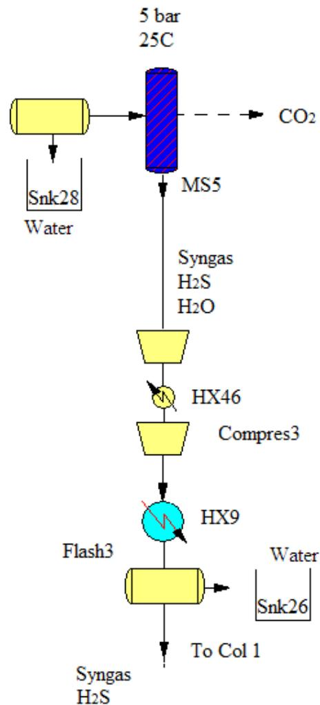
Figure 3.- Scheme for the removal of H<sub>2</sub>S and CO<sub>2</sub>
