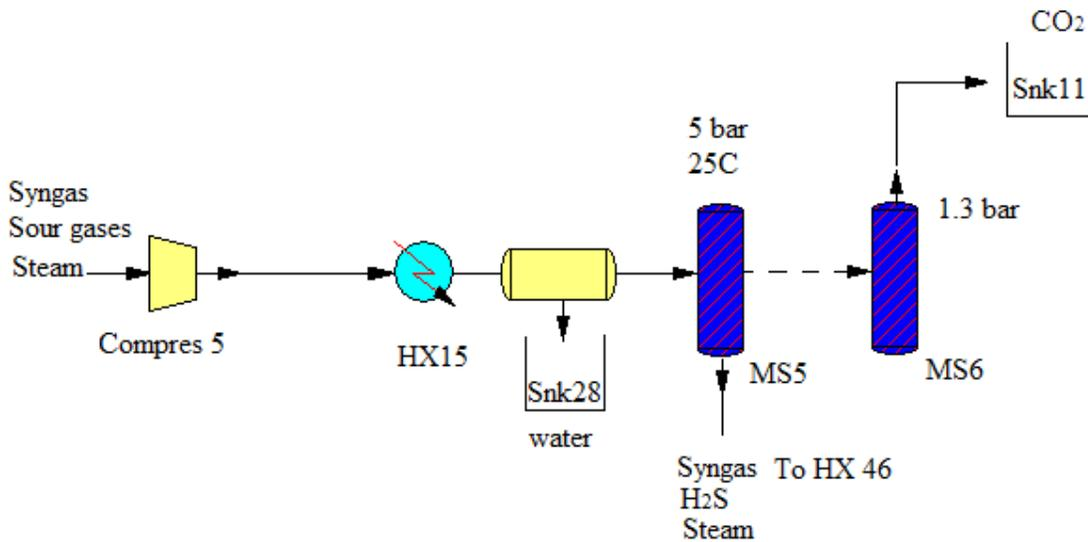
Figure 2.- PSA system for the removal of CO<sub>2</sub>
