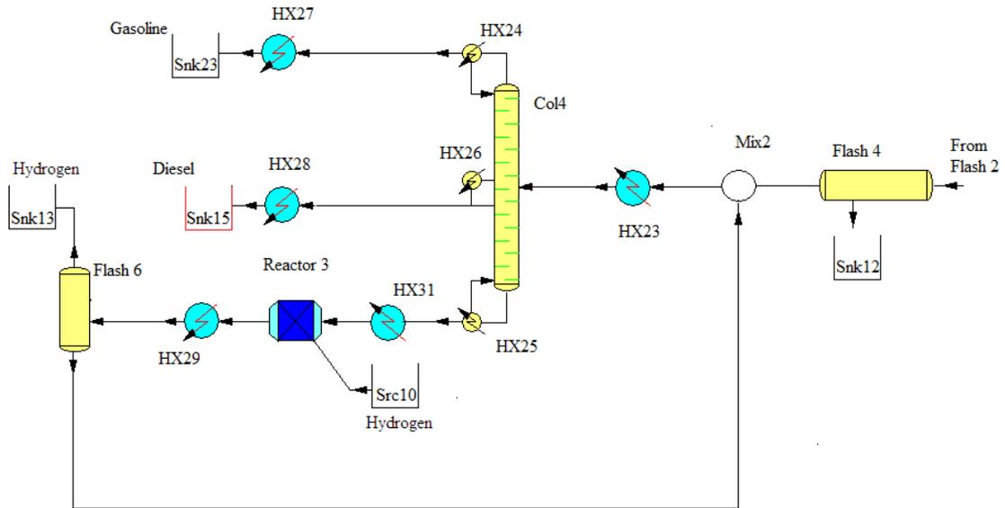
Figure 9.- Diesel and gasoline fractionation
