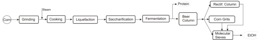
Fig. 8.1 Block diagram for corn based ethanol
