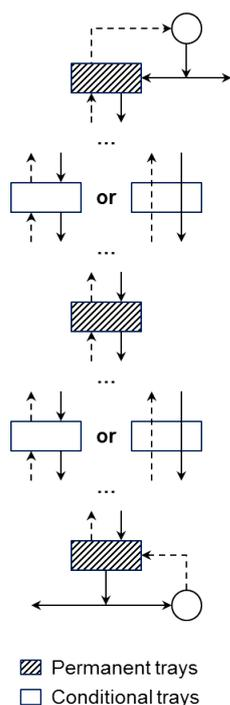
Figure 15: Illustration of the GDP model representation for tray by tray design of distillation columns.
