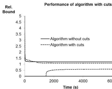
Figure 10: Performance of the algorithm,, for layout-optimization of screening systems, with and without cutting planes when dropping the nonlinear constraints in the master problem.
