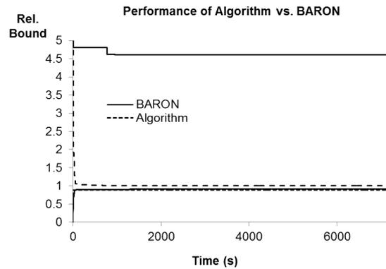
Figure 12: Performance of BARON and the complete algorithm, for reactor-separator process superstructure, using polyhedral envelopes for the linear relaxation in the master problem.
