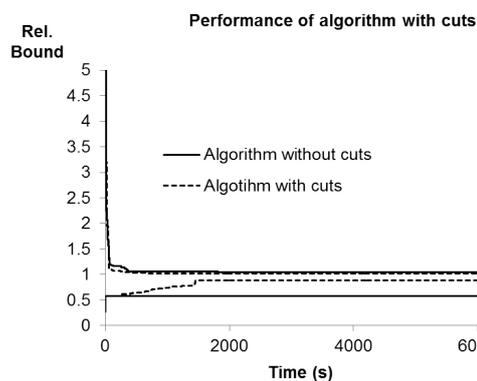
Figure 14: Performance of the algorithm, for reactor-separator process superstructure, with and without cutting planes when dropping the nonlinear constraints in the master problem.
