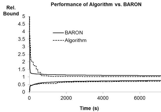
Figure 8: Performance of BARON and the complete algorithm, for layout-optimization of screening systems, using polyhedral envelopes for the linear relaxation in the master problem.
