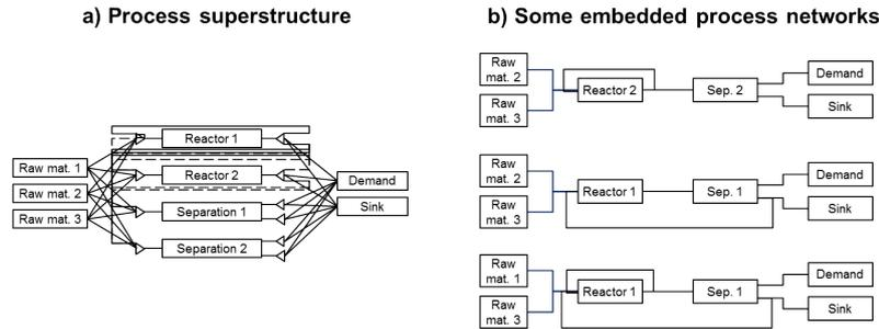
Figure 11: Illustration of process superstructure with two reactors and two separators.
