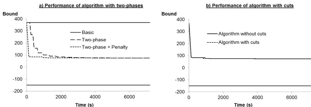
Figure 16: Performance of the algorithm, for reactor-separator process superstructure, with a) Two-phase enhancement and b) cutting planes.
