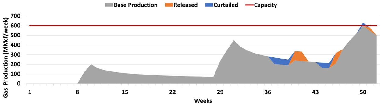
(c) Optimal production of gas, including curtailment, from the wells assuming mobilization costs are three times the original estimate.
