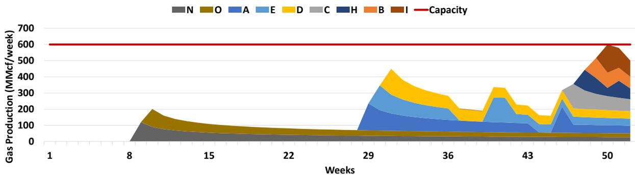
(c) Optimal production of gas from the wells assuming mobilization costs are three times the original estimate.
