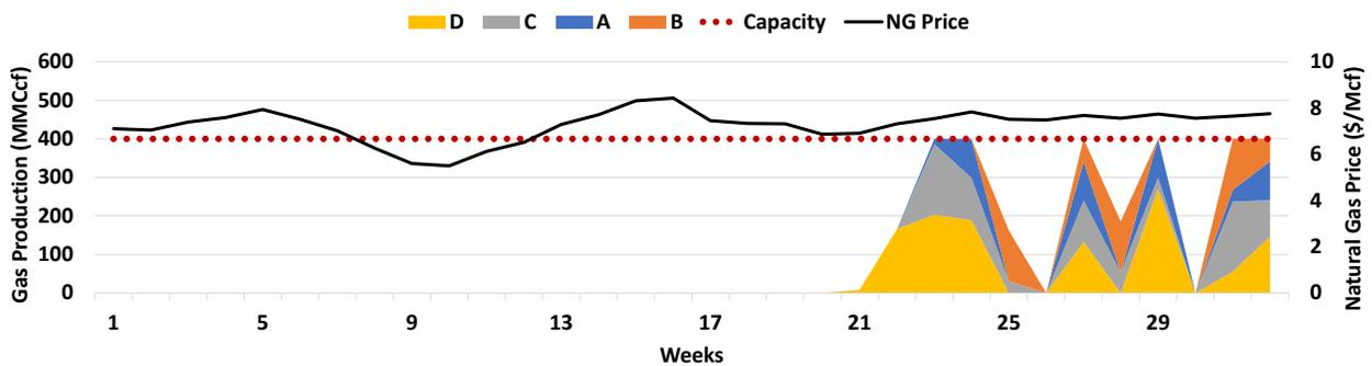
(b) Optimal production of gas from the wells at the illustrative pad.
