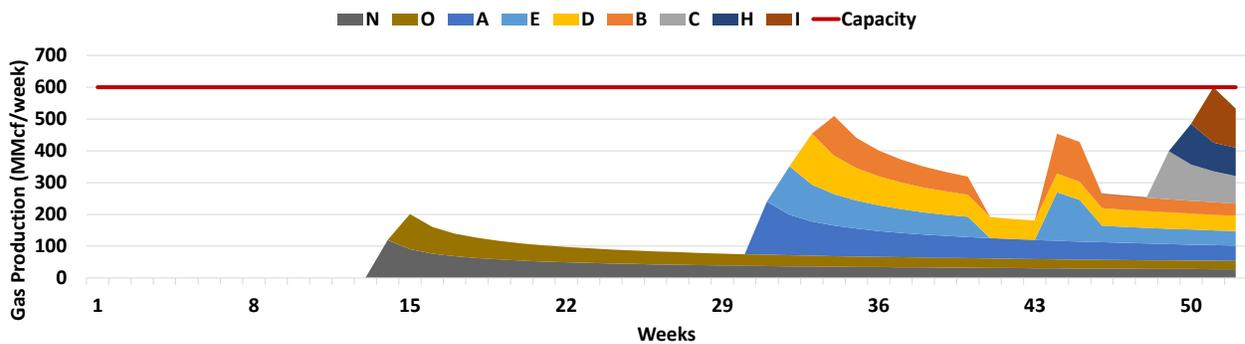
(b) Optimal production of gas from the wells assuming mobilization costs are two times the original estimate.
