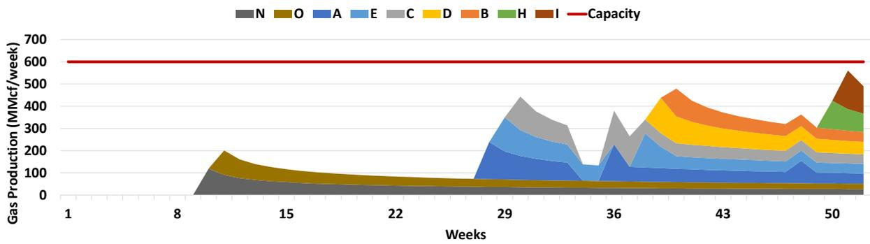
(b) Optimal production of gas from the wells using the original estimate of mobilization costs.
