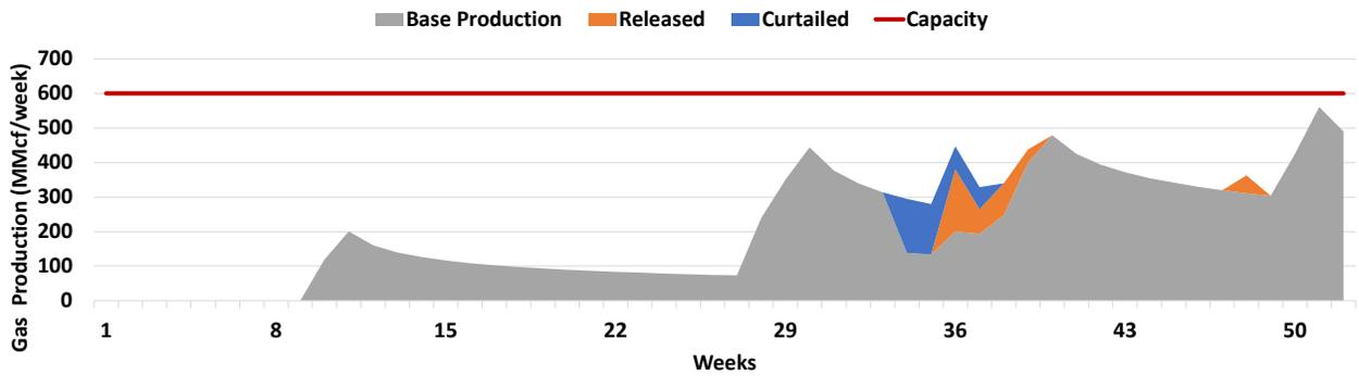
(a) Optimal production of gas, including curtailment, from the wells using the original estimate of mobilization costs.
