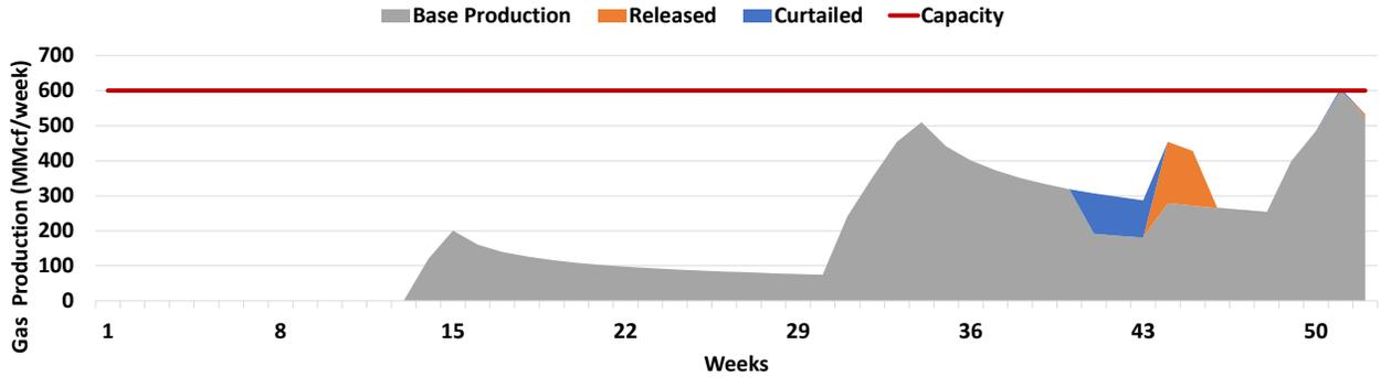
(b) Optimal production of gas, including curtailment, from the wells assuming mobilization costs are two times the original estimate.
