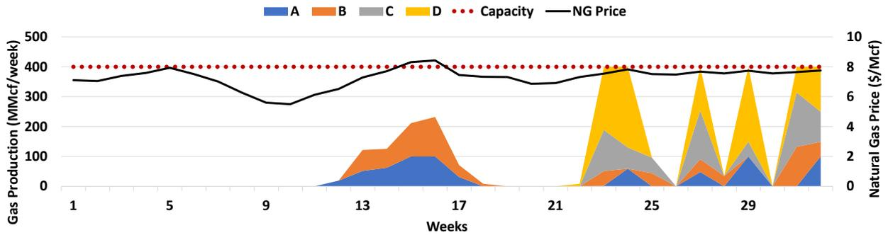
(b) Optimal production of gas from the wells at the illustrative pad.
