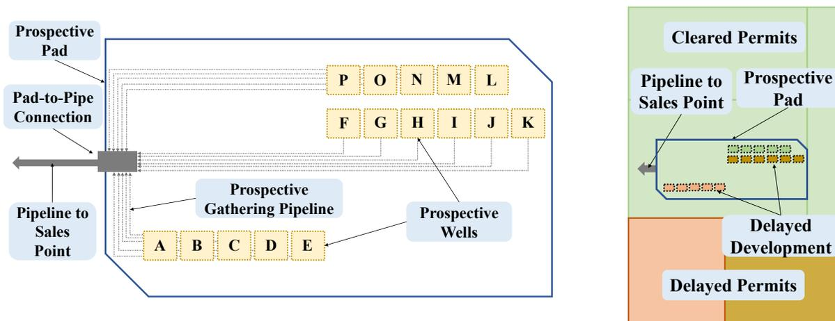
(a) Pad-level diagram of the prospective pad, including prospective wells and their associated gathering pipelines.
