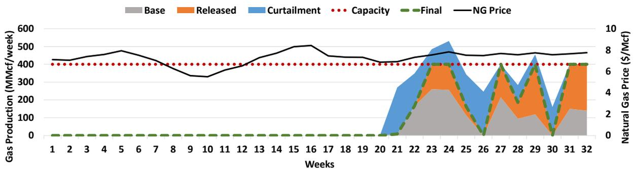
(c) Optimal production of gas, including curtailment, at the illustrative pad.
