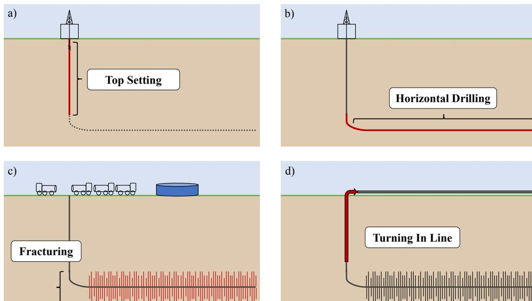
Figure 1: The four operations necessary to develop a well to completion: a) top setting, b) horizontal drilling, c) hydraulic fracturing, and d) turning in line.
