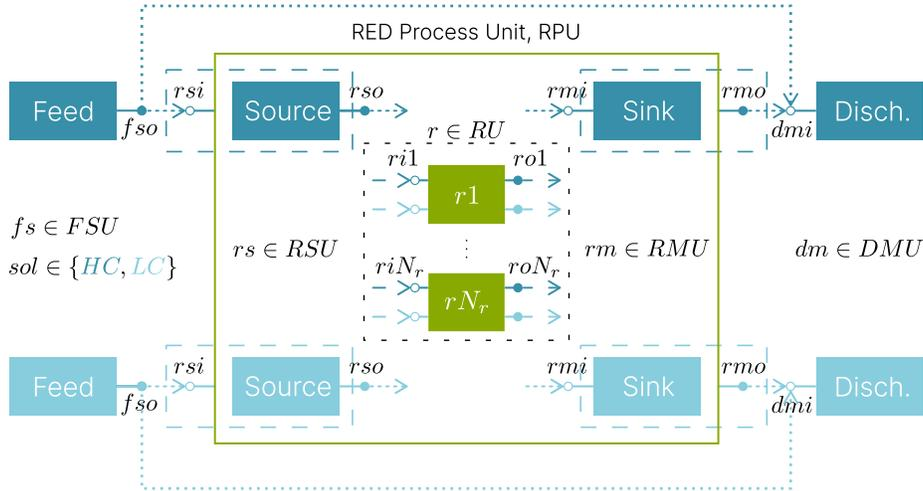
**Figure 1:** Superstructure for the RED process with: the set of high (HC) and low-salinity (LC) feed ( $f_s \in FSU$ ) and discharge ( $dm \in DMU$ ) units; the set of source ( $rs \in RSU$ ) and sink ( $rm \in RMU$ ) units and the set of candidate RED units ( $r \in RU$ ) embedded in the RED Process unit (RPU); the set of inlet and outlet ports; and the set of streams or links between outlet-to-inlet port pairs. Adapted from [8].
