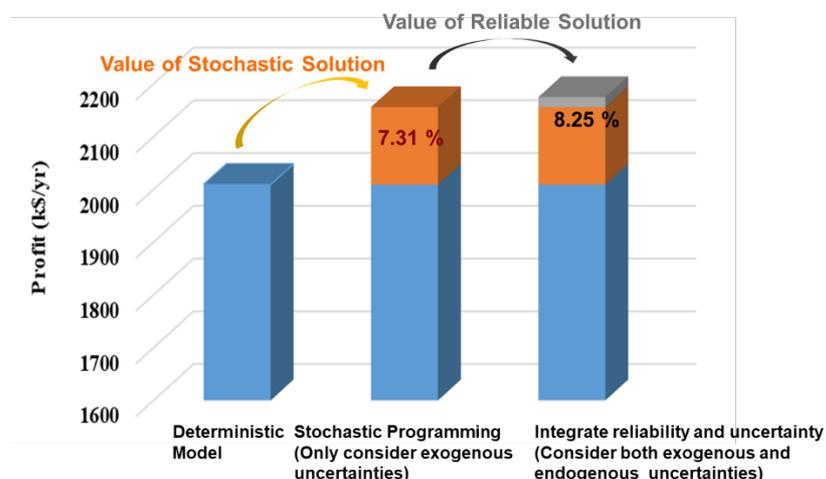
**Fig. 7.** Comparison of the total annualized profit for three different optimization models in terms of VSS and VRS (Methanol synthesis process).
