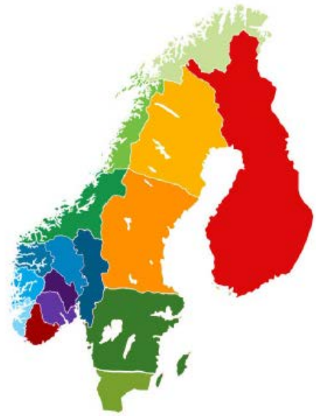
Figure 1: New hydro regions as modeled in the HBV and SDDP models. Notice that the hydro regions for Norway are not identical to the price regions (NO1-5).
