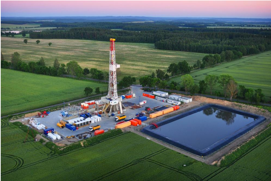
Figure 2. A representative shale well site showing a drilling rig and an adjacent water storage (Image source: https://www.kontextwochenzeitung.de/ueberm-kesselrand/78/gorleben-am-bodensee-981.html )
